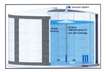
Note: To the left, for illustrative purposes only, is a schematic diagram of a THM Removal System. This quotation is only the in-tank water-handling equipment, namely the Floating Spray Nozzle equipment, any Tank Mixing equipment required and the Ventilation System.
